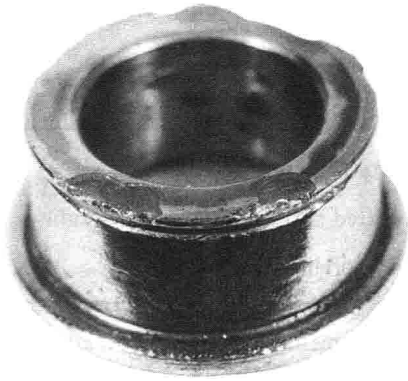
Cracked inner race
