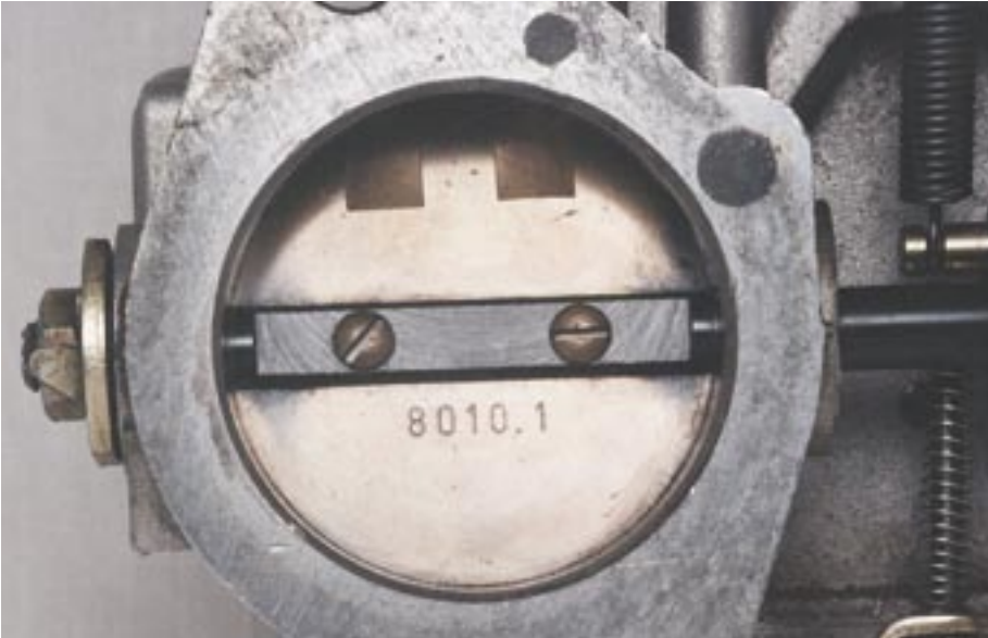
Dellorto butterflies with the progression hole sweep slots and the numbers clearly visible.
