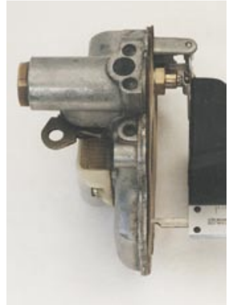
Dellorto floats being set at 15mm when the needle is just seating.
