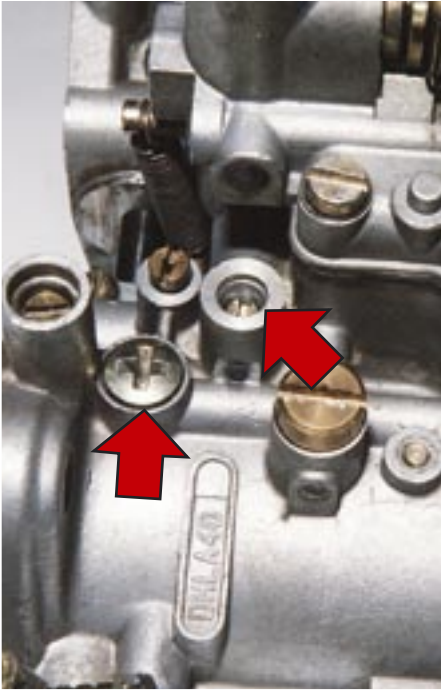
On this Dellorto carburettor the progression hole plug (A) has a Phillips head, and the idle by-pass adjustment screw is in a tower (B).
