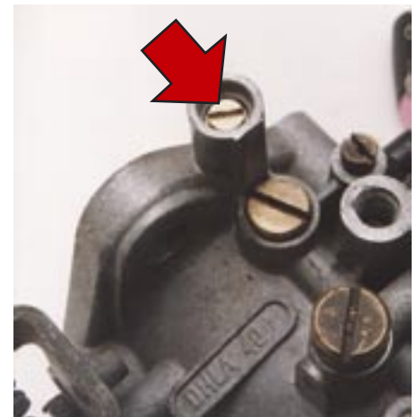
Dellorto carburettors with towers have very fine threaded idle mixture adjustment screws which frequently seize solid and the screwdriver slot gets damaged.
