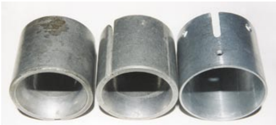
Dellorto chokes, 40mm version on the left, 45mm centre and 48mm right.
