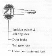
Ignition key can be inserted and removed at the "LOCK" position only.
