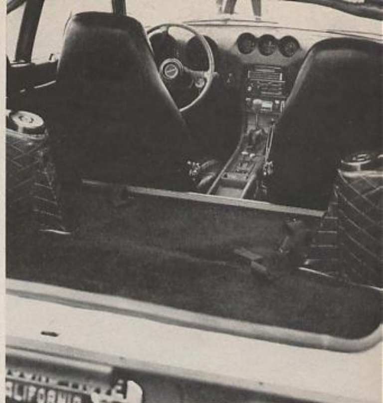
Instrumentation is complete, well arranged and readable except for distance to the small instruments from driver's eye. Rear suspension intrudes into rear cargo area but capacity is still generous; spare tire lives in well beneath floor.
