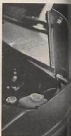
A nice touch borrowed from Porsche (below) is this rubber flap that flops out when the gasoline filler door is opened.
