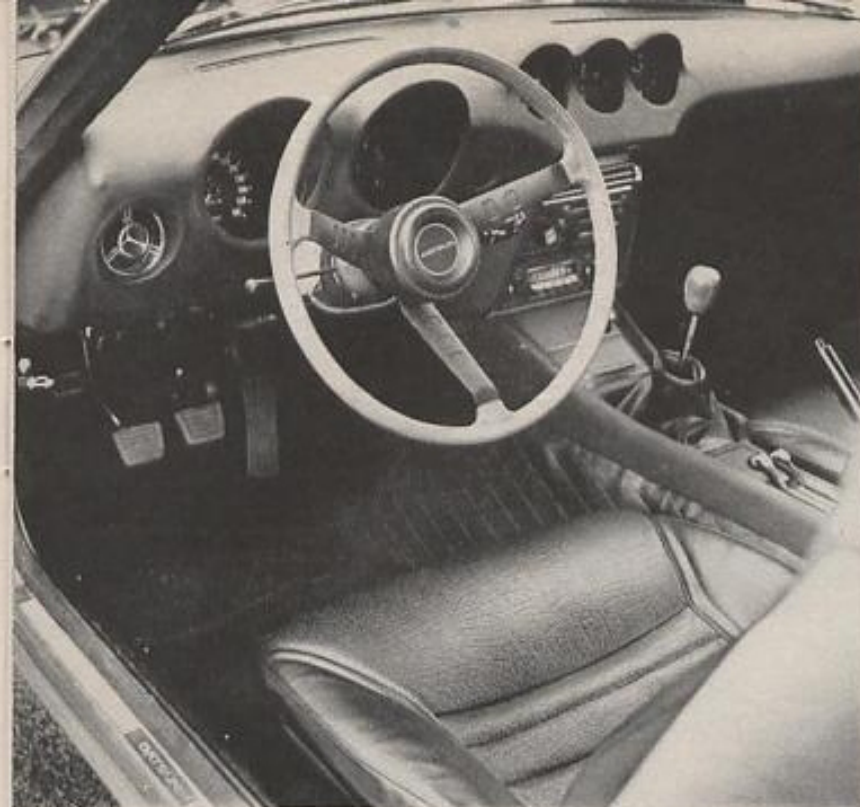
Instrumentation is complete, well arranged and readable except for distance to the small instruments from driver's eye. Rear suspension intrudes into rear cargo area but capacity is still generous; spare tire lives in well beneath floor.
