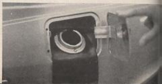
A nice touch borrowed from Porsche (below) is this rubber flap that flops out when the gasoline filler door is opened.
